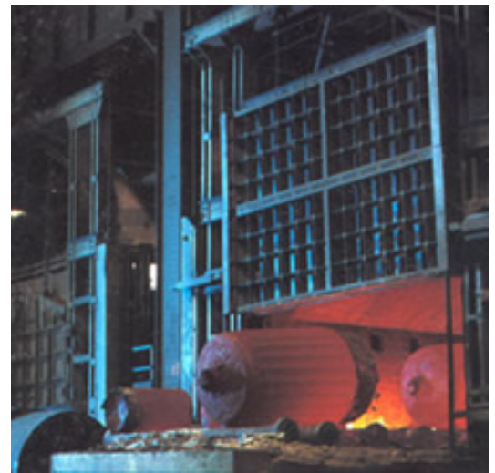
Ellwood Quality Steel Large Car-Bottom Furnace
